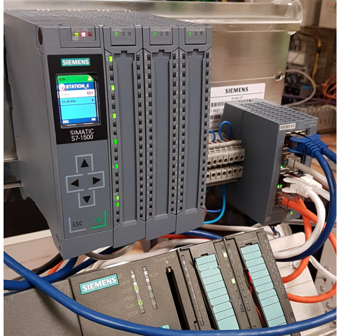
Our new training rigs now feature the Siemens S7-1500 PLC connected to a range of sensors and networked systems so that we can teach the latest techniques to implement Industry 4.0 methodology. Visit our website for full details.
